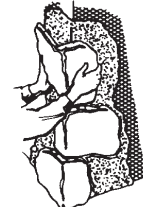
Figure 8 Apply corners—alternating long and short legs in the opposite directions.
