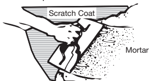
Figure 5 Apply mortar using a plasterer's trowel.
